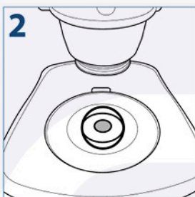
2 Put a specimen on the stage plate
