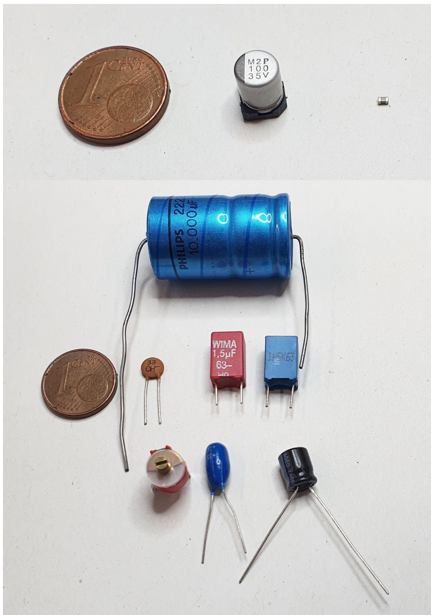
Fig. 34: types of capacitors
