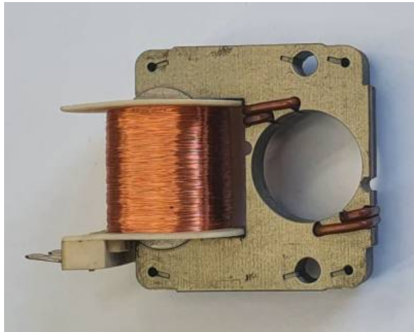
Fig. 25: Core of a shaded Pole Motor
