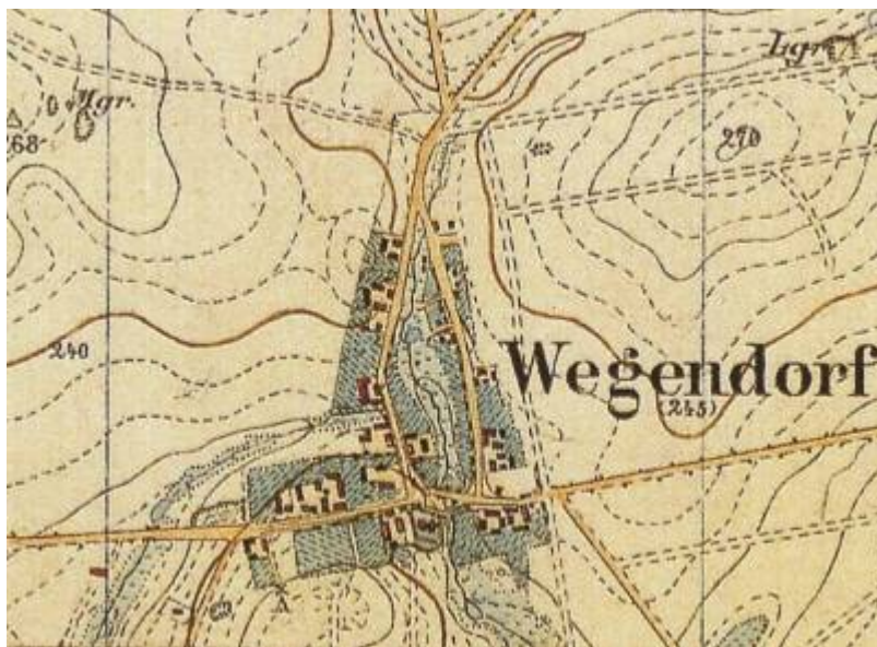
Fig. 13: Indicating elevation contours on a map
