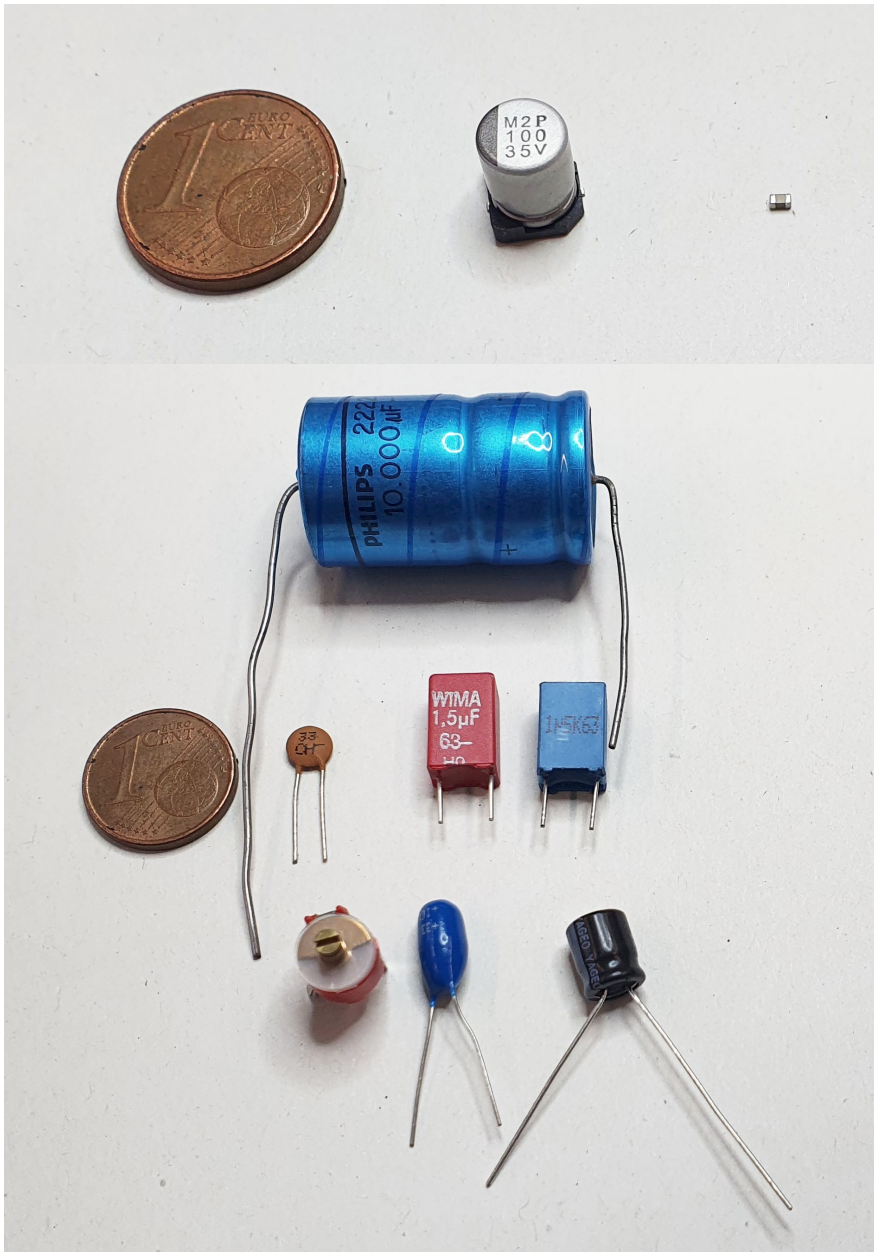
Fig. 2: types of capacitors
