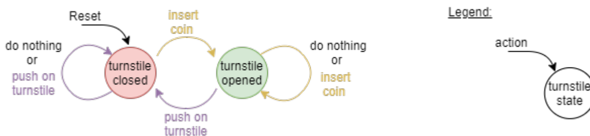
Fig. 12: State Transition Diagram of the Entrance Control for Toilets
