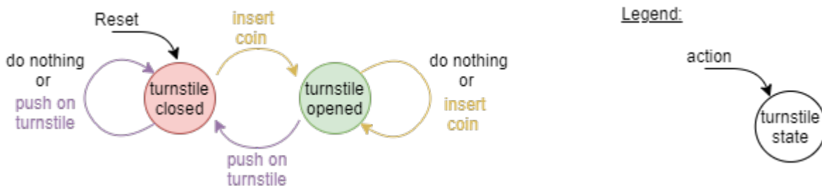
Fig. 12: State Transition Diagram of the Entrance Control for Toilets
